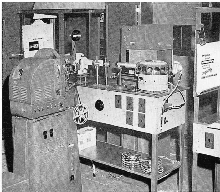
FIG. 18. Each one of the TK-20 Iconoscope Film Chains has a TP-16 16mm Film Projector and two slide-projector inputs.
