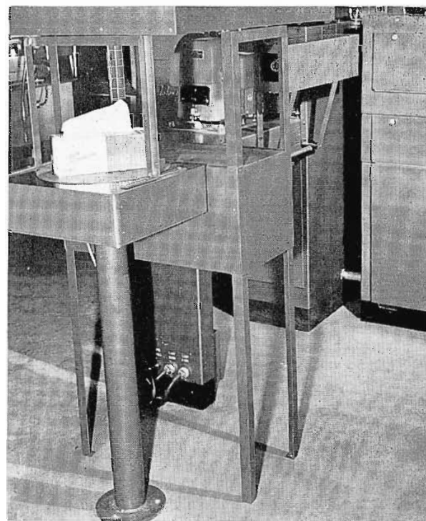
FIG. 20. This arrangement is employed for producing opaques, or live commercials using 3-V System. Note the product on the turntable (left)—optical setup is mounted on brackets and can be seen to the left of the TP-6 16mm projector.
