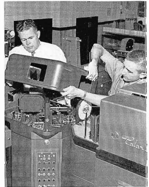
FIG. 2. Final check is made on 3-V color film chain multiplexer. An input for opaques has also been provided in this equipment.
