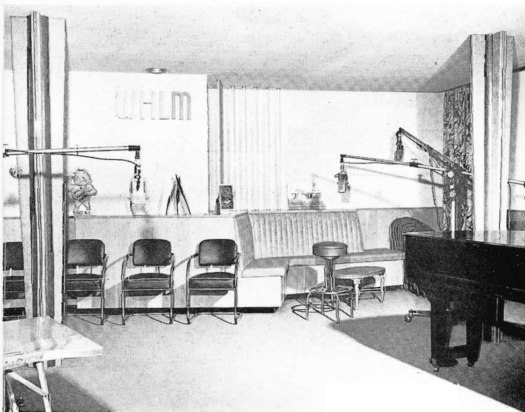
FIG. 2. One of the spacious, tastefully decorated WHLM studios. Large enough to accommodate a reasonable-size audience. The studio's irregular shape prevents multiple reflections . . . improves acoustics.
